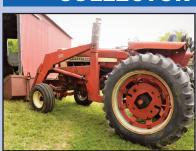
International Harvestor Hydro 70, Diesel tractor, 15.5 X 38 Rubber With 1500 Loader 1975 - Ser# 2680017U009897 Less than 300 hours on complete engine overhaul
